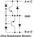
NOTE: All GND terminals should be connected to ground.
