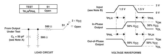
NOTES: A. C<sub>L</sub> includes probe and jig capacitance.
