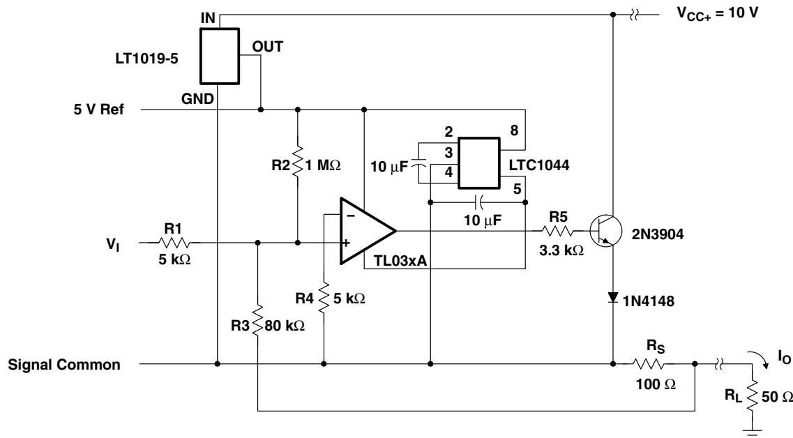
Figure 67. Two-Wire 4-mA to 20-mA Current Loop
