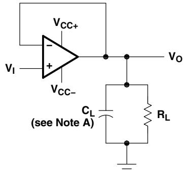
NOTE A:  $C_L$  includes fixture capacitance.
