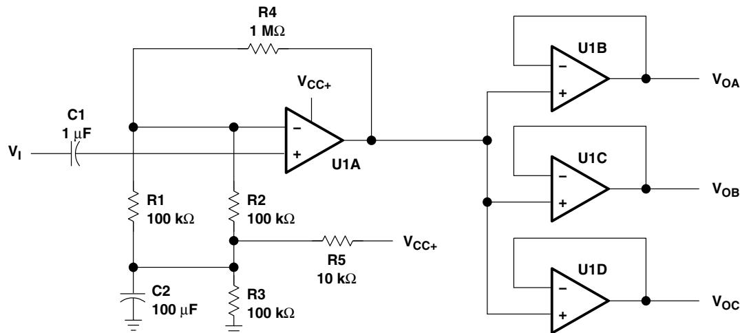
NOTE A: U1A through U1D = TL03x;  $V_{CC+} = 5\ V$
