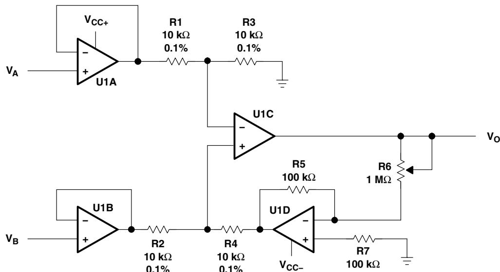
NOTE A: U1A through U1D = TL03x;  $V_{CC\pm} = \pm 15$  V
