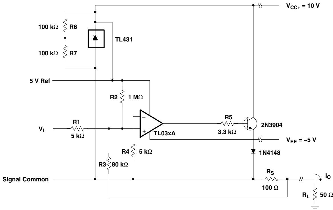
Figure 66. Three-Wire 4-mA to 20-mA Current Loop
