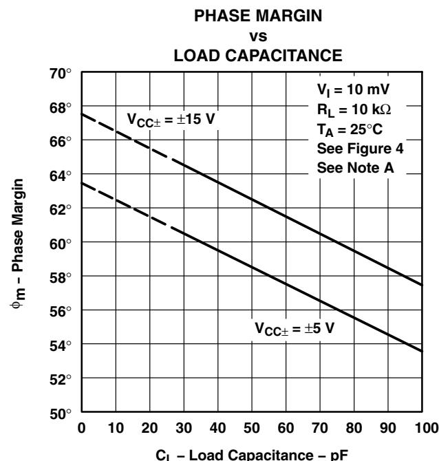
NOTE A: Values of phase margin below a load capacitance of 25 pF were estimated.
