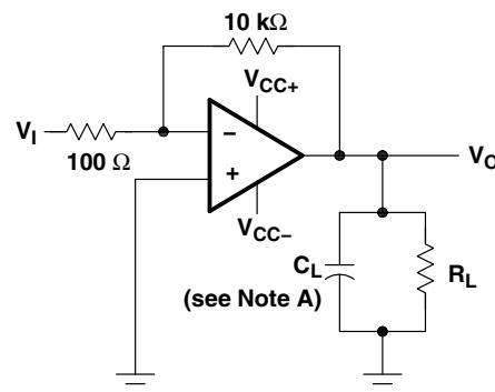
NOTE A:  $C_L$  includes fixture capacitance.
