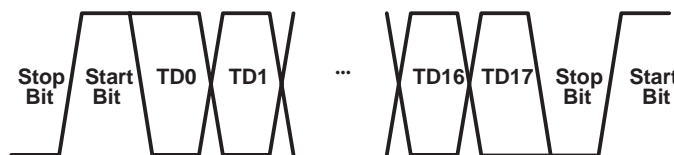
Figure 3. Serial Output Data Stream with Start and Stop Bit
