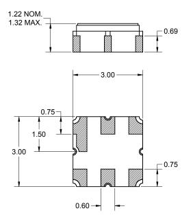
Dimensions shown are nominal in millimeters All tolerances are  $\pm 0.15$ mm except overall length and width  $\pm 0.10$ mm
