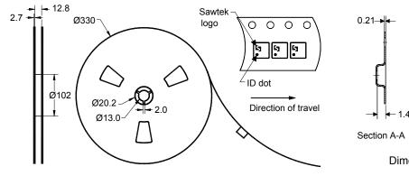
Dimensions shown are nominal in millimeters Packaging quantity: 5000 units/reel
