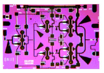
The TriQuint TGA1073B-SCC is a three stage HPA MMIC design using TriQuint's proven 0.25 um Power pHEMT process. The TGA1073B is designed to support a variety of millimeter wave applications including point-to-point digital radio and LMDS/LMCS and Ka band satellite ground terminals.
