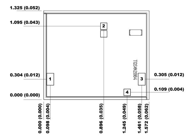
Units: millimeters (inches) Thickness: 0.100 (0.004) Chip edge to bond pad dimensions are shown to center of bond pad Chip size tolerance: +/- 0.051 (0.002)
