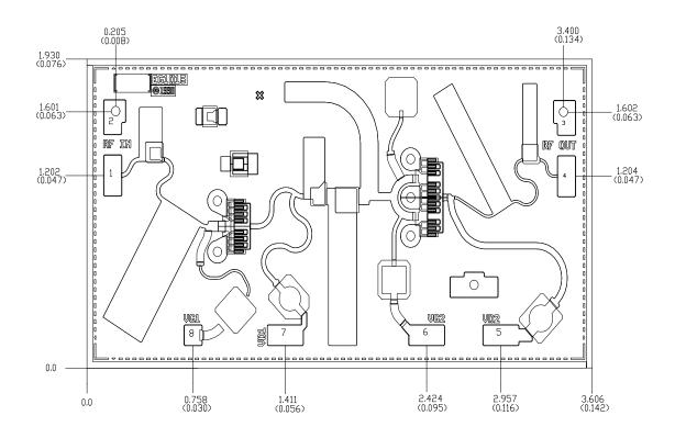
Units: millimeters (inches) Thickness: 0.1016 (0.004)
