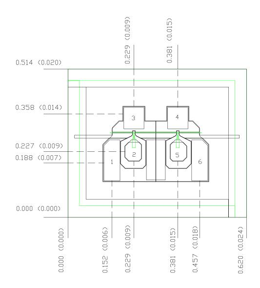
Units: millimeters (inches) Thickness: 0.1016 (0.004)
