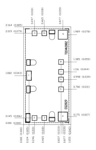
Units: millimeters (inches) Thickness: 0.100 (0.004) Chip edge to bond pad dimensions are shown to center of bond pads. Chip size tolerance: +/- 0.0508 (0.002) GND IS BACKSIDE DF MMIC Bond Pad #1 (RF\_A) 0.105  $\times$  0.205 (0.004  $\times$  0.008) Bond Pad #2 (VC3) 0.105  $\times$  0.105 (0.004  $\times$  0.004) Bond Pad #3 (VC4) 0.105  $\times$  0.105 (0.004  $\times$  0.004)
