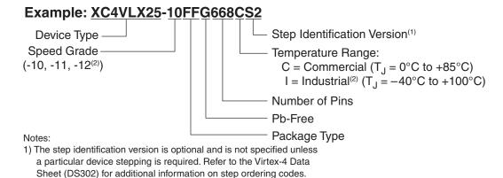
Figure 1: Virtex-4 FPGA Ordering Information
