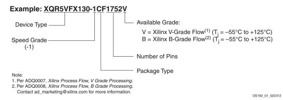
Figure 1: Virtex-5QV FPGA Ordering Information
