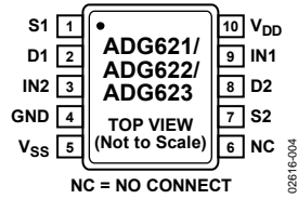
Figure 4. 10-Lead MSOP (RM-10)
