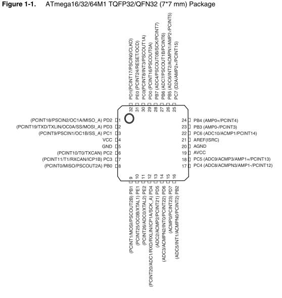
Note: On the engineering samples (Parts marked AT90PWM324), the ACMPN3 alternate function is not located on PC4. It is located on PE2.
