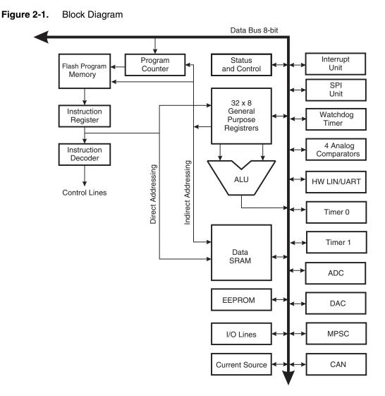
The AVR core combines a rich instruction set with 32 general purpose working registers. All the 32 registers are directly connected to the Arithmetic Logic Unit (ALU), allowing two independent registers to be accessed in one single instruction executed in one clock cycle. The resulting architecture is more code efficient while achieving throughputs up to ten times faster than conventional CISC microcontrollers.
