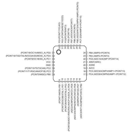
Note: On the first engineering samples (Parts marked AT90PWM324), the ACMPN3 alternate function is not located on PC4. It is located on PE2.
