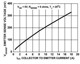
Figure 2. Emitter Sense Voltage vs. Collector to Emitter Current
