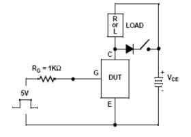
Figure 20.  $t_{ON}$  and  $t_{OFF}$  Switching Test Circuit
