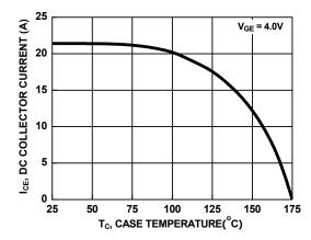
Figure 11. DC Collector Current vs. Case Temperature
