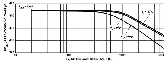
Figure 17. Break 8 own Voltage vs. Series Gate Resistance
