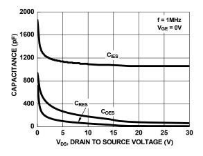
Figure 15. Capacitance vs. Collector to Emitter Voltage
