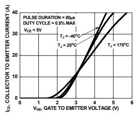
Figure 10. Transfer Characteristics
