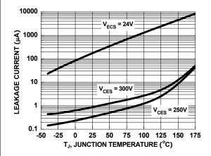
Figure 13. Leakage Current vs. Junction Temperature
