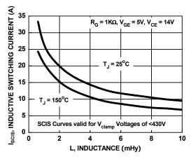
Figure 4. Self Clamped Inductive Switching Current vs. Inductance
