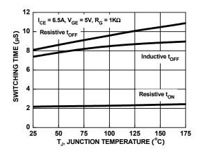
Figure 14. Switching Time vs. Junction Temperature
