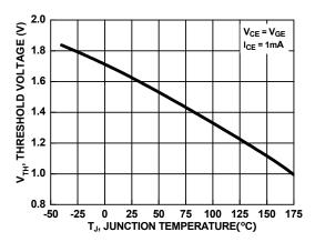
Figure 12. Threshold Voltage vs. Junction Temperature
