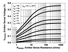
Figure 1. Emitter Sense Voltage vs. Emitter Sense Resistance
