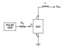
Figure 19. Inductive Switching Test Circuit
