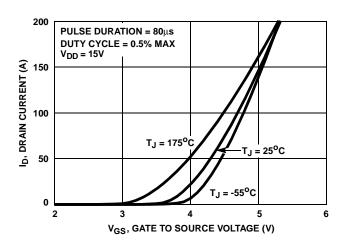
FIGURE 7. TRANSFER CHARACTERISTICS
