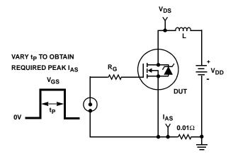
FIGURE 14. UNCLAMPED ENERGY TEST CIRCUIT
