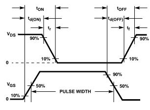
FIGURE 19. SWITCHING TIME WAVEFORM
