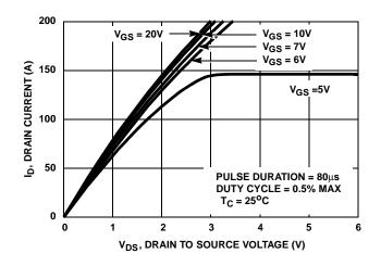
FIGURE 8. SATURATION CHARACTERISTICS
