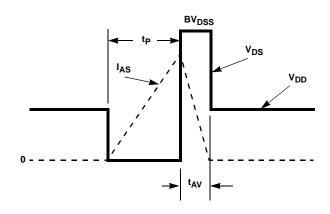
FIGURE 15. UNCLAMPED ENERGY WAVEFORMS
