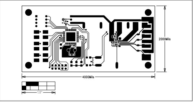
Figure 4. MAX8822 EV Kit PCB Layout—Component Side
