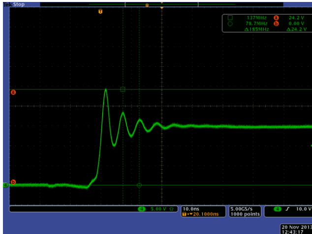
Figure 5. Switch Node Original Ring Waveform
