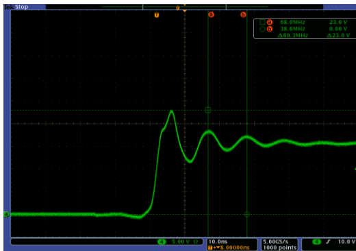
Figure 10. V_{SW} with Parallel 2.2 nF Capacitor Added
