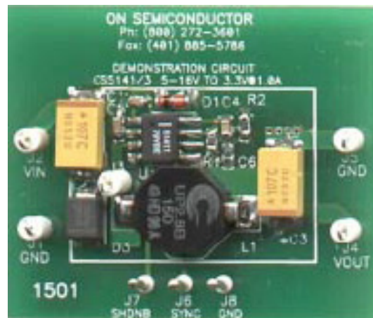
Figure 1. CS51411/3 Demonstration Board
