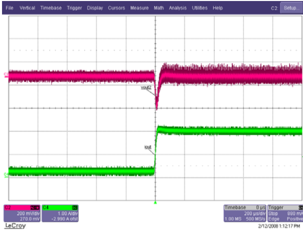
Figure 11. Load Transient – V_{out2} ( V_{in} = 12\text{ V} , I_{out} = 200\text{ mA} \rightarrow 2\text{ A} \rightarrow 200\text{ mA} ) (CH1 = V_{out2} , CH4 = I_{out2} )
