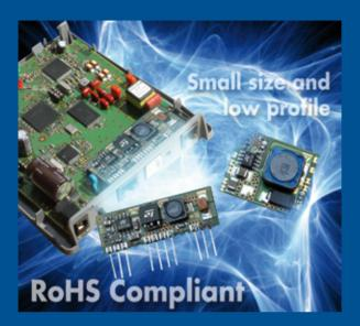
The GSR family provides the complete voltage-regulation function in a proven circuit architecture and high-efficiency design. Based on an ST device, the non-isolated GSR gives you accurate voltage regulation in a variety of applications.
