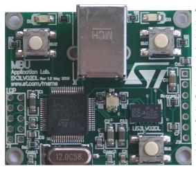
The **EK3LV02DL** will help you in evaluating the LIS3LV02DL 3-Axis - $\pm 2g/\pm 6g$  Digital Output Low Voltage Linear Accelerometer MEMS accelerometers. The kit implements a typical application which enables the user to acquire the acceleration data sensed by the LIS3LV02DL product. In details, the signal measured by the sensor are read by the microcontroller of the ST7 family mounted on the board and they are sent to a PC for further processing via USB link
