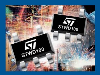
The new STWD100 is a standalone watchdog circuit that improves system reliability by monitoring the system for software code execution errors. When the watchdog input detects a transitional edge, the internal watchdog timer clears and restarts, then begins counting again. If the watchdog timer exceeds the watchdog timeout period, the active-low output asserts for the watchdog pulse period to alert the system of a fault condition.
