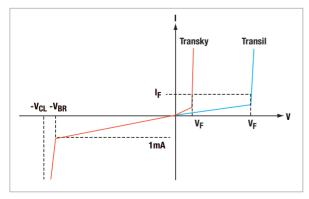
Expanding its EOS and ESD protection portfolio, **STMicroelectronics** is now releasing its 5V and 12V low forward voltage Transil protection devices, the Transky SMTY5.0A and SMTY12A.
