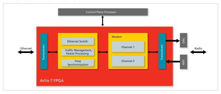
Artix-7 FPGAs offer the system integration and signal processing capabilities needed to extend network coverage via mobile backhaul units. These devices offer the right mix of logic density, IP, and DSP resources to integrate backhaul solutions comprised of packet processing, traffic management, timing and synchronization blocks as well dual high-speed radio channel.
