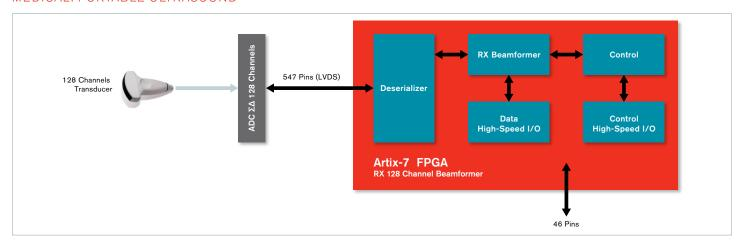
Designers can deploy a fully programmable 128-channel portable ultrasound implementation that scales up to 196 or 256 channels for high-end cart solutions or down to 64 or 32 channels for hand-held form factors.
