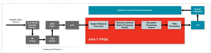
The Artix-7 FPGA delivers the industry's most integrated Type-1 single-chip cryptography (SCC) solution for superior, secure SWaP-C results. Extensive DSP resources allow for waveform processing capacity to integrate both modem and cryptographic engine on a single chip.
