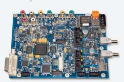
• The logiCRAFT 6 Development Board is part of the base platform of a complete Hybrid Instrument Cluster Targeted Design Platform. The associated fully functional reference design includes stepper motor gauge control, dual TFT displays (including a HUD), and Rear Camera input/display. Image distortion correction is also implemented for both HUD and Rear Camera.
