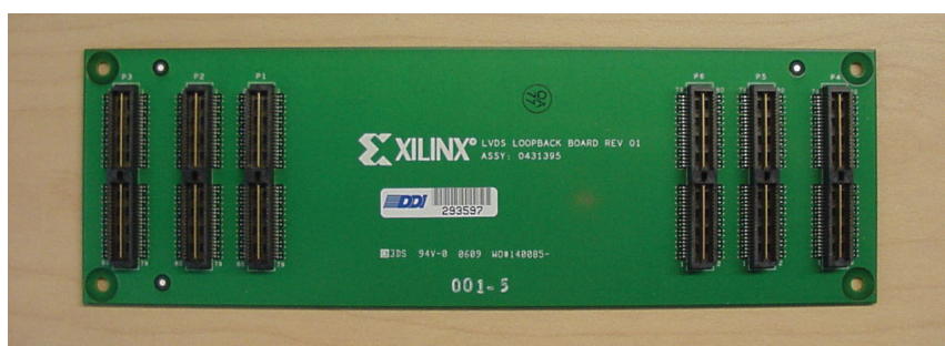
Figure B-1: Xilinx LVDS Loopback Board
