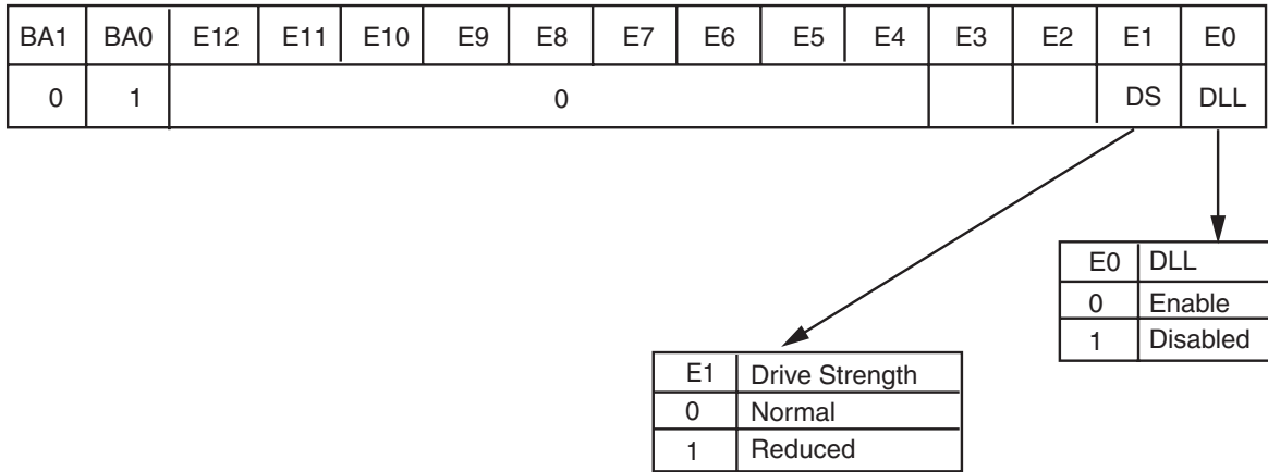
Figure 2: Extended Mode Register for DDR400
