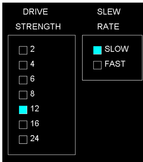
Figure 5: Drive Strength and Slew Rate Boxes from IOB Block
