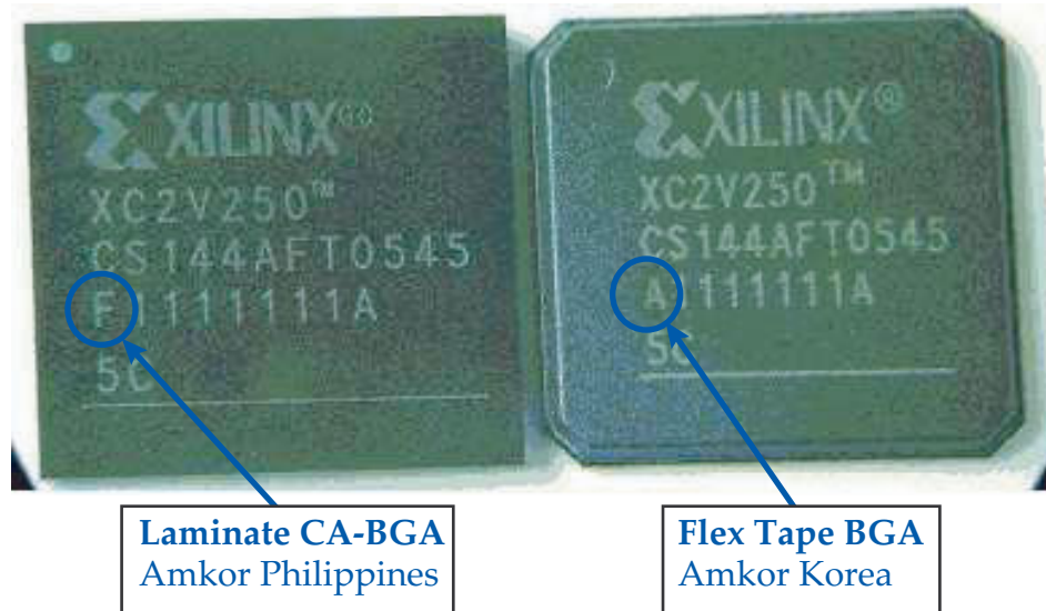
Figure 1: Package Top Mark Showing Assembly Site Code
