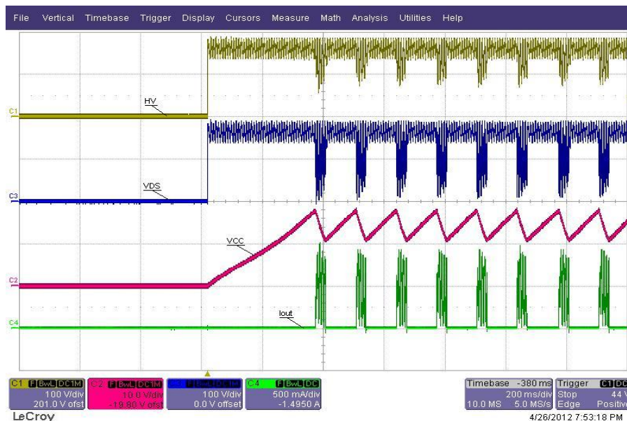
Figure 15 Waveforms during start-up with output short-circuited: Input voltage at HV pin (C1, yellow), Vcc voltage (C2, red), MOSFET drain voltage (C3, blue), and output current (C4, green)
