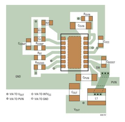
Figure 7. Example of Power Component Layout for DFN Package. Because of the Similar Pinout, MSE Package Layout is Similar
