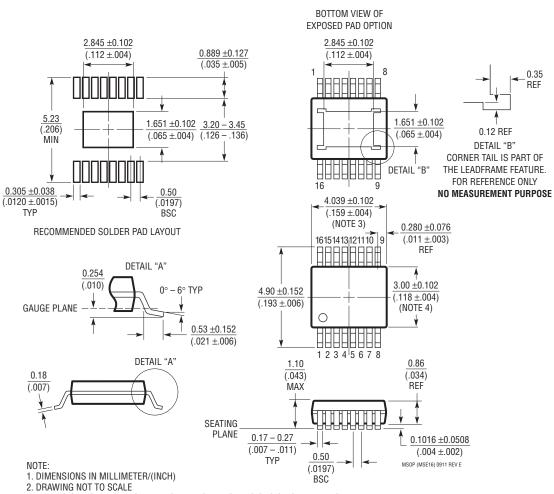
MSE Package 16-Lead Plastic MSOP, Exposed Die Pad (Reference LTC DWG # 05-08-1667 Rev E)
