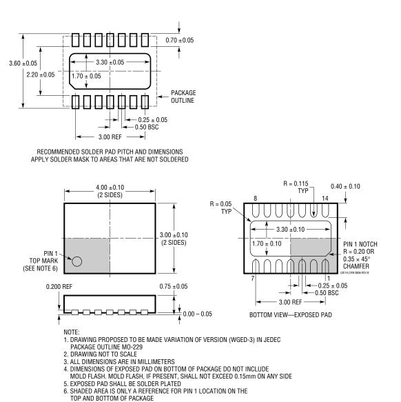
DE Package 14-Lead Plastic DFN (4mm × 3mm) (Reference LTC DWG # 05-08-1708 Rev B)
