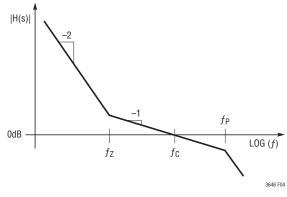
Figure 4. Bode Plot of Regulator Loop
