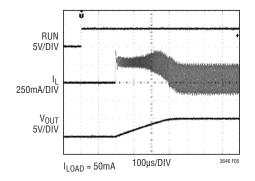
Figure 5. Start-Up Waveform
