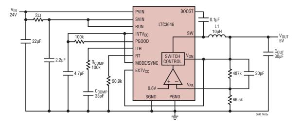
24V Input to 5V Output at 1MHz Frequency and  $\text{EXTV}_{\text{CC}}$
