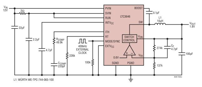
12V to 1.8V Output with 400kHz External Sync
