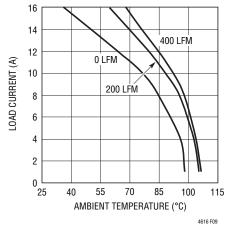
Figure 9. 5V<sub>IN</sub> to 3.3V<sub>OUT</sub> with No Heat Sink
