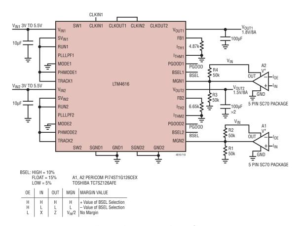
Figure 18. Typical 3V to  $5.5V_{\mbox{\scriptsize IN}},$  to 1.8V, 1.5V Outputs
