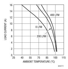
Figure 11. 5V<sub>IN</sub> to 3.3V<sub>OUT</sub> with BGA Heat Sink
