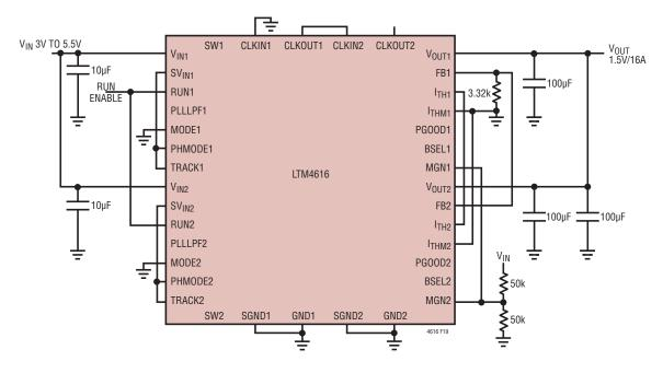
Figure 19. LTM4616 Two Outputs Parallel, 1.5V at 16A Design
