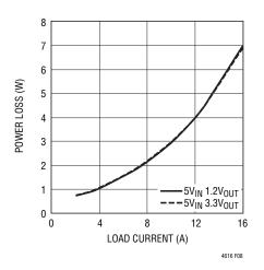
Figure 8. 1.2V, 3.3V Power Loss
