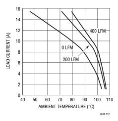
Figure 12.  $5\mbox{V}_{\mbox{\scriptsize IN}}$  to 1.2 $\mbox{V}_{\mbox{\scriptsize OUT}}$  with BGA Heat Sink
