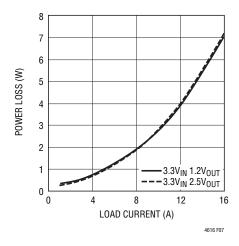
Figure 7. 1.2V, 2.5V Power Loss
