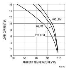
Figure 16.  $3.3\mbox{V}_{\mbox{\scriptsize IN}}$  2.5 $\mbox{V}_{\mbox{\scriptsize OUT}}$  with BGA Heat Sink
