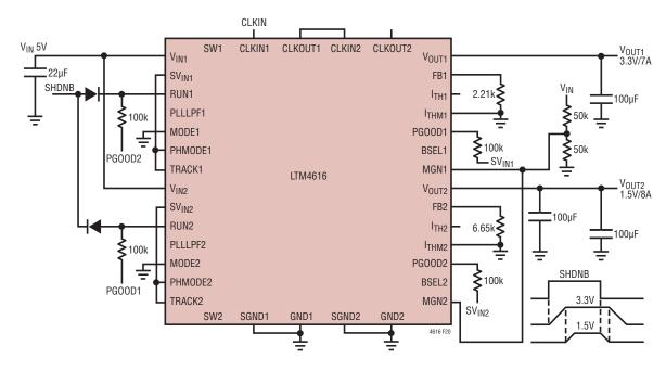
Figure 20. LTM4616 Output Sequencing Application
