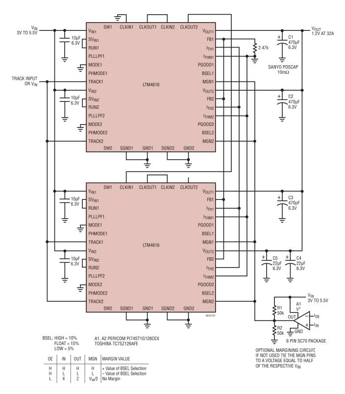
Figure 21. Four Phase in Parallel, 1.2V at 32A
