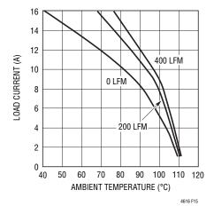
Figure 15. 3.3  $V_{\mbox{\scriptsize IN}}$  1.2  $V_{\mbox{\scriptsize OUT}}$  with BGA Heat Sink
