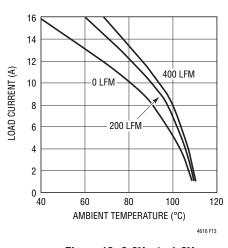
Figure 13.  $3.3\mbox{V}_{IN}$  to  $1.2\mbox{V}_{OUT}$  with No Heat Sink
