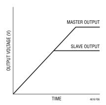
Figure 6. Output Voltage Coincident Tracking
