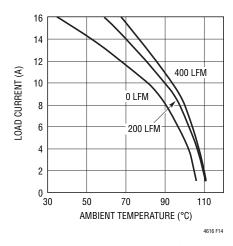
Figure 14.  $3.3\mbox{V}_{IN}$  to  $2.5\mbox{V}_{OUT}$  with No Heat Sink
