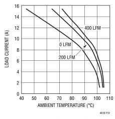
Figure 10.  $5V_{IN}$  to 1.2 $V_{OUT}$  with No Heat Sink
