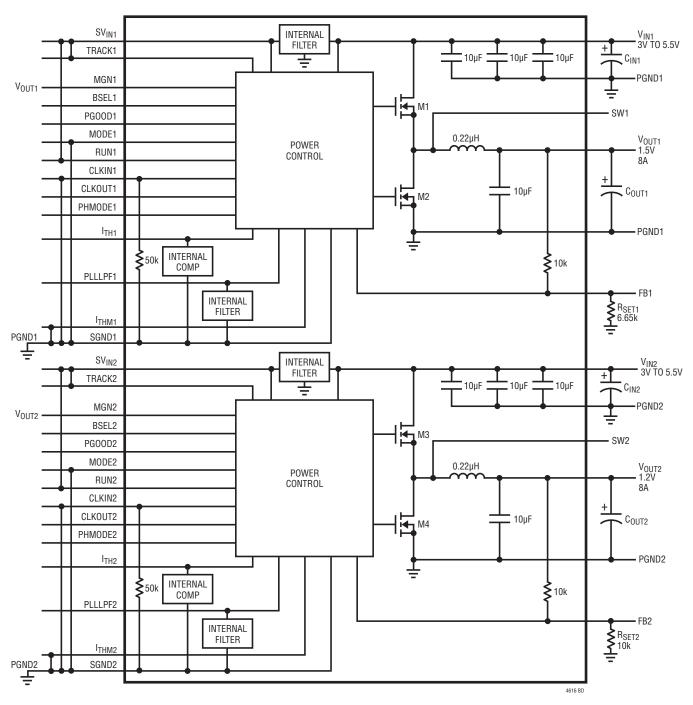
Figure 1. Simplified LTM4616 Block Diagram
